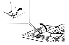
**2** Gently pull the jammed printout *up and out.* The printout may be jammed either within the fax (*left*, below), or in the output tray (*right*, below).
